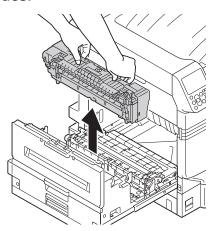
If the paper winds around the decal roller, remove the decal unit by turning the thumbscrews at both ends of the decal unit to the left, and remove the paper.
