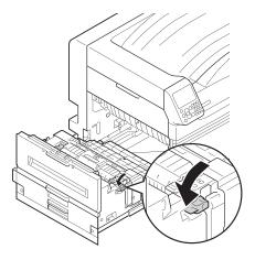
14 Put the exit unit back into the printer.
