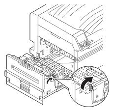
Hold the fuser unit handle with both hands, and remove it onto a flat surface.
