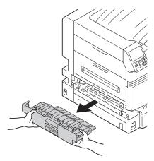
Remove the remaining paper from the printer.
