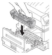
11 Push down the fuser unit's lock lever (blue).
