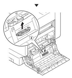
Insert the new paper feed rollers (②), and firmly insert up to inside along the notch.
