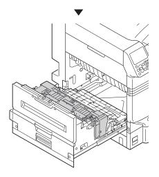
13 Push down the fuser unit's lock lever (blue).
