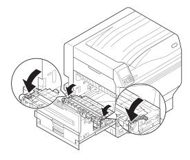
12 Set the fuser unit to the label position of the exit unit by holding its handle with your hands.
