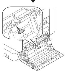
Pinch the claws (two places) and remove the separator (4). Open Section B, and remove the separation rollers (3).
