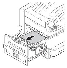
If the paper tip is not visible, pull up the fuser unit's lock lever (blue).
