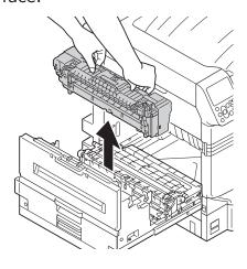
Raise the jam release lever of the fuser
