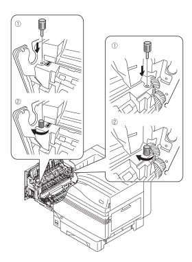
10 Hold the knob, pull up the transfer roller unit, lift the paper guide, and remove the remaining paper.
