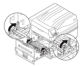
Remove the transfer roller unit by holding its label part (blue).
