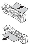
If the paper winds around the decal roller, remove the decal unit by turning the thumbscrews at both ends of the decal unit to the left, and remove the paper.
