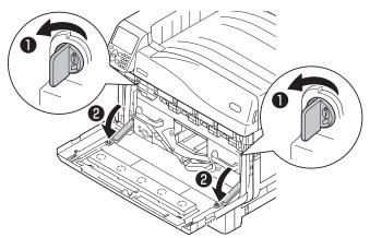
Hold the handle and pull out the belt unit, hold the left-right label part (blue) and remove the belt unit.
