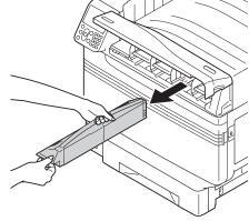
Remove the new toner cartridge from its packaging, and shake it vertically and horizontally.
