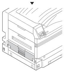
Lift opener (①) of the exit unit, and pull out the exit unit.
