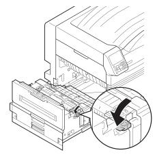
Put the exit unit back into the printer.
