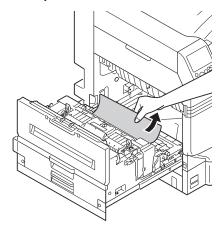
Push down the fuser unit's jam release lever (blue).
