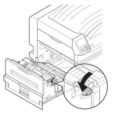
12 Put the exit unit back into the printer.
