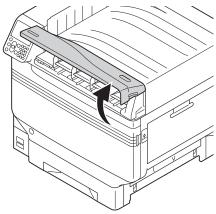
Check the position of toner cartridge to be replaced, via the label letters and color.
