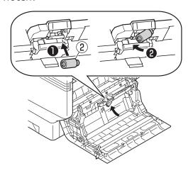
10 Insert the new feed rollers (1) in the axial, and firmly insert up to inside while rotating them.
