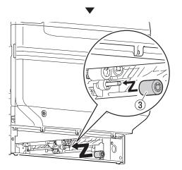
**9** Check that no paper feed roller is missing.
