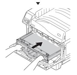
10 Raise the belt unit left/right lock lever, rotate the lock lever knob (blue) to the right and lock it.
