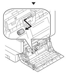
Wipe off the dirt on paper feed rollers (1) with the moist soft cloth.
