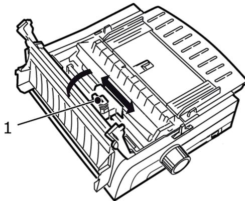
2. Swing the used ribbon cartridge up off the printhead, lift it out, and discard it.
