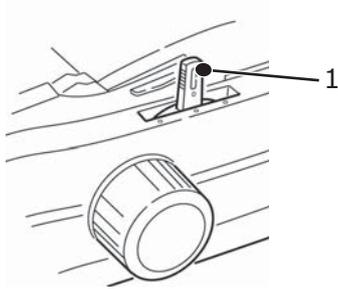
5. Adjust the paper guides (1) for the size of paper you are using, then place a sheet of paper in the sheet guide.
