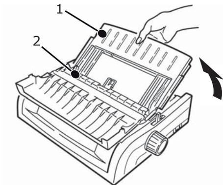
3. Pivot the sheet guide forward and gently rest it against the roller assembly (2). If you push the sheet guide too hard against the roller assembly, it may dislodge it. If it does, be sure to reset the roller assembly before continuing.
