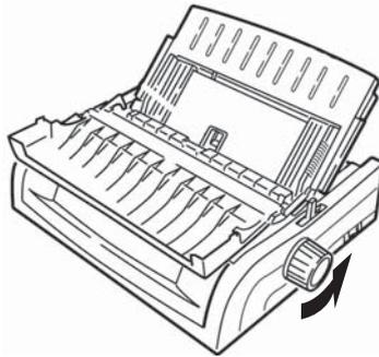
3. Open the access cover (1) and remove the pull-up roller assembly (2).
