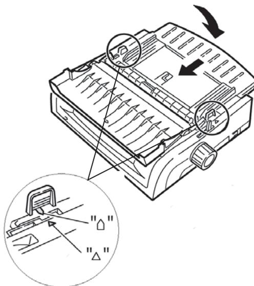
11. Place the wire guide in the sheet guide on the pull-up roller assembly.
