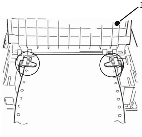
5. Lower the sheet guide, then install the pull-up roller assembly and close the access cover.
