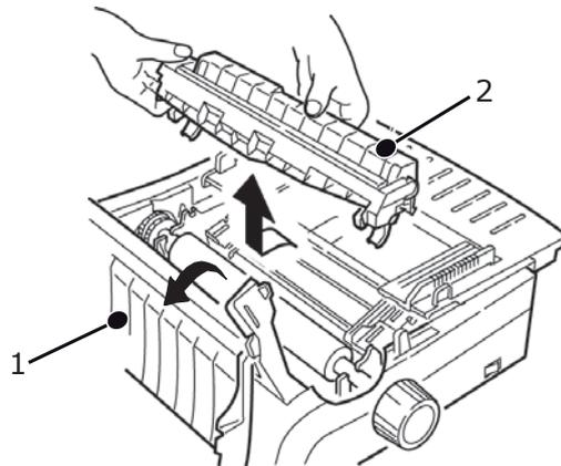
4. Lift the sheet guide (1) and reload paper. Make sure you lock the tractor covers.
