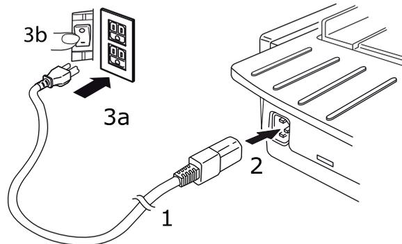
3. Connect the power cable to a 220/240 V A/C power outlet (3a) and switch on the outlet power (3b).
