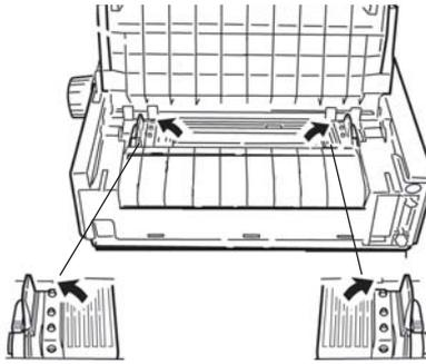
7. Place continuous forms paper on the first two pins of either tractor.
