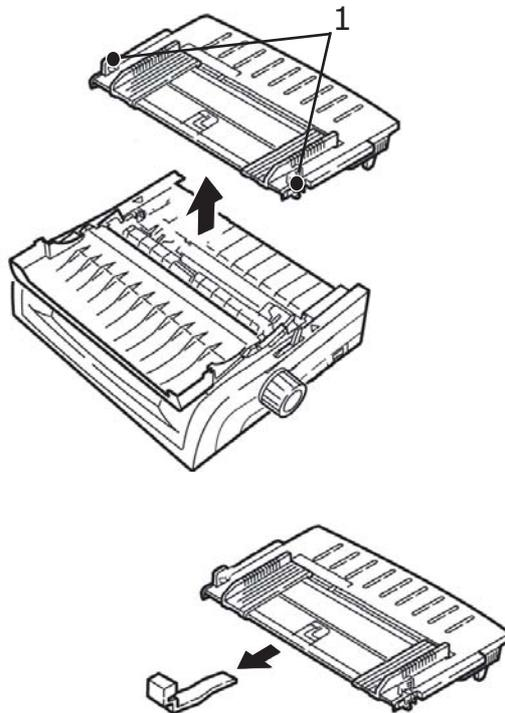
5. Reinstall the sheet guide: insert the clips on either side of the separator into the notches marked with a triangle, then press down to secure the separator in place.
