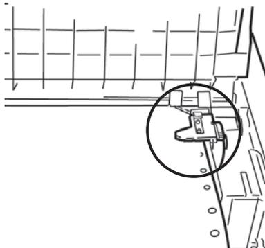
9. Adjust the left tractor until the holes in the paper are centered on the pins then lock the lever and close the left tractor cover.
