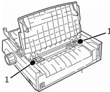
5. Open the lock levers (1) and move the right tractor (as viewed from the back of the printer) to the reference mark (2) matching the width of the paper you are loading. Then close the lock lever on the right tractor:
