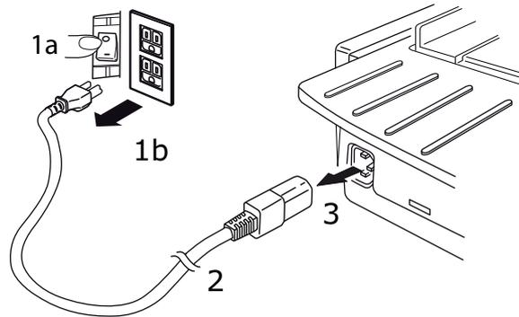
3. Unplug the power cable connector (2) from the printer (3).
