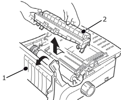
4. Use a clean, dry cloth to dust around the carriage shaft and platen. Remove any loose bits of paper.
