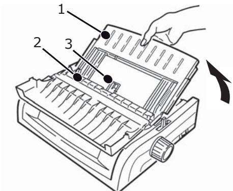
3. Adjust the paper feed guides (1) for the width of the paper, then place a sheet of paper in the separator. The paper will feed into the printer.
