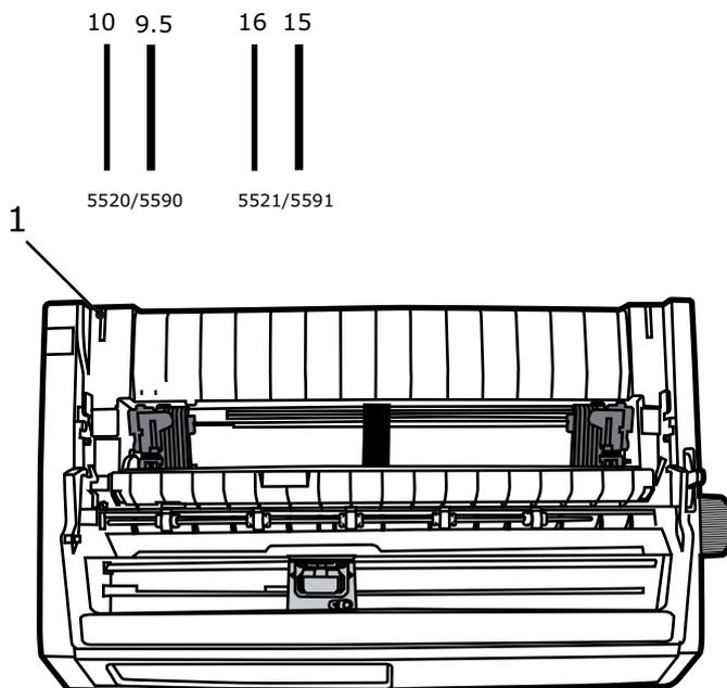
5. Open the tractor covers and place continuous forms paper on the first two pins of either tractor, then close the left tractor cover.
