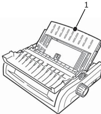
3. Pivot the wire feed guide into the sheet guide.
