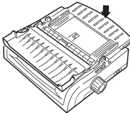
3. Swing the wire feed guide over onto the pull-up roller.
