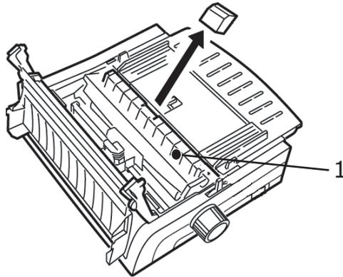
4. Use the tabs (1) to lift and remove the sheet guide, then remove the shipping restraint.
