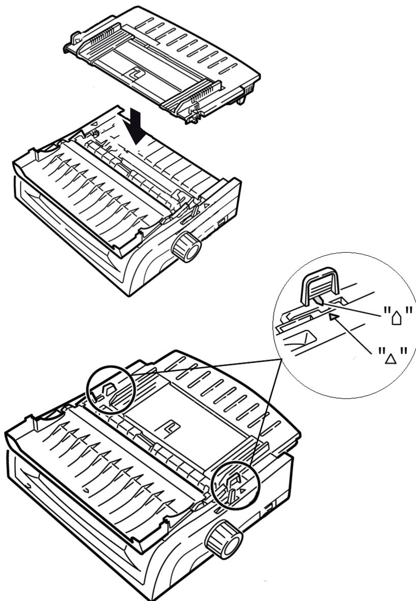
8. Place the wire guide (1) in the sheet guide on the pull-up roller assembly.
