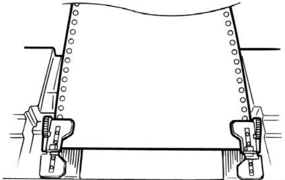
6. Use the platen knob to draw the quadruple-thick page around the platen. This brings out jammed pieces of paper.
