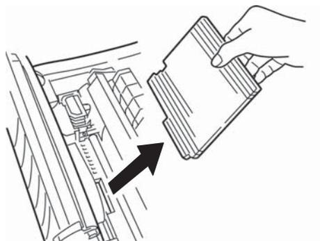
3. Remove the shipping restraint from the pull-up roller assembly (1).
