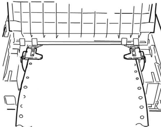
9. Install the sheet guide, then install the pull-up roller assembly and close the access cover.
