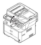
11 Press the top cover open button (7) and open the top cover.
