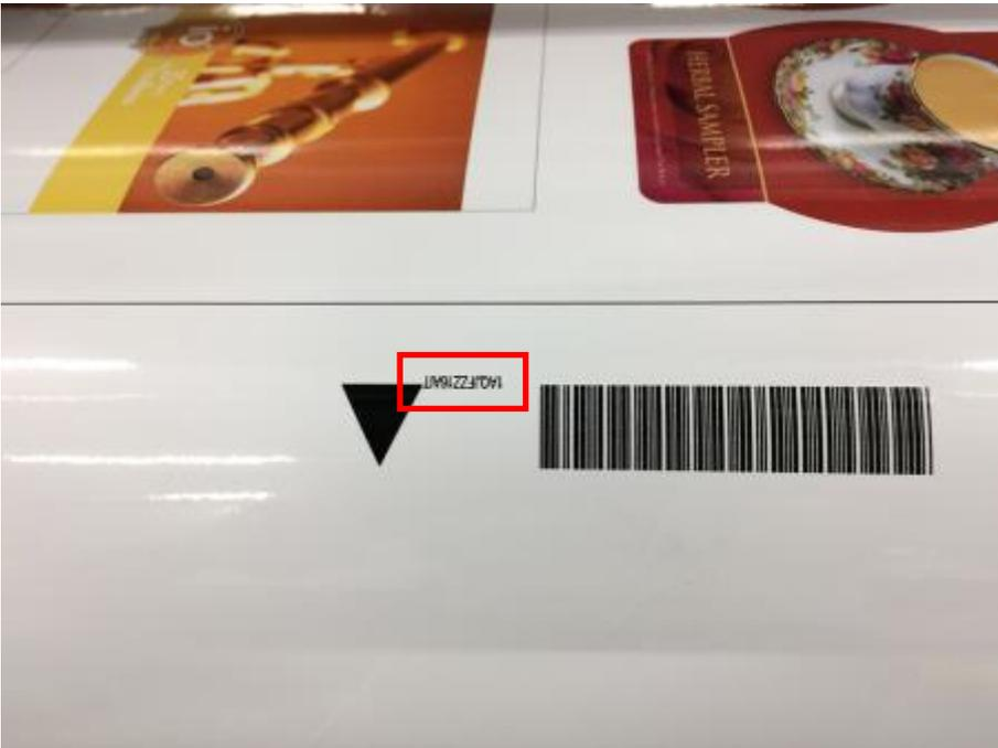
Use the arrow buttons of the cutting plotter to move the cutting tool inside the right-hand registration mark on the front.
