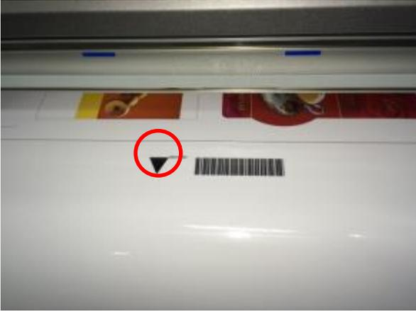
Check the name of the cut data file printed next to the triangles. The name is "1AQFZZ16AIT" in this example.
