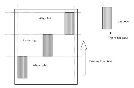
Printing positions are changed as follows by the *alignment* parameters in 90-degree-to-the-left orientation.
