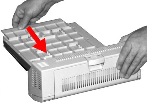
**6.** Push the duplexer back into the printer.
