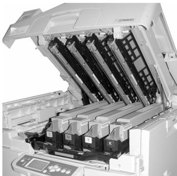
3. Use the lens cleaner supplied with the toner cartridges (or a clean, soft cloth) to gently clean the LED heads (1).
