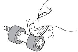
4. Turn the short tab of the feed roll to the right and slowly push it onto the shaft of the paper tray.
