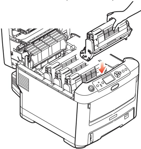
9. Lower the top cover but do not press down to latch it closed yet. This will protect the drums from excessive exposure to room lighting while you check the remaining areas for jammed sheets.
