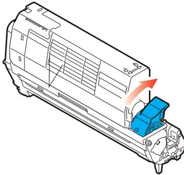
10. Holding the complete assembly by its top center, lower it into place in the printer, locating the pegs at each end into their slots in the sides of the printer cavity.
