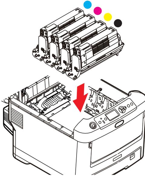
Holding the complete assembly by its top center, lower it into place in the printer, locating the pegs at each end into their slots in the sides of the printer cavity.
