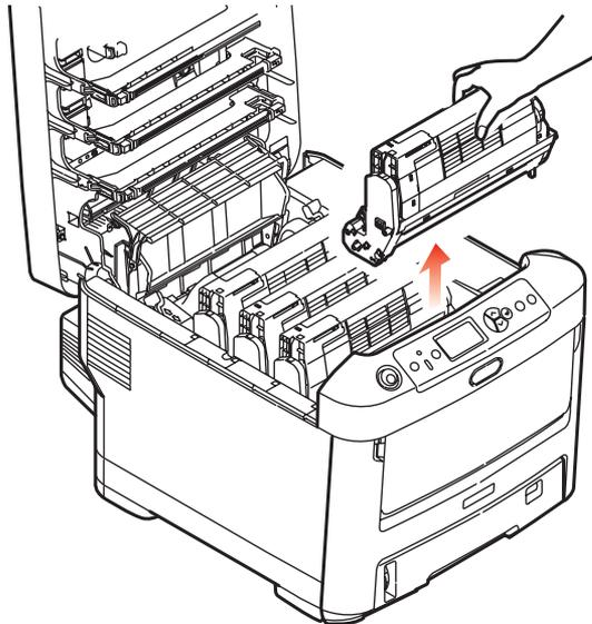
5. Put the assembly down gently onto a piece of paper to prevent toner from marking your furniture and to avoid damaging the green drum surface, and cover.
