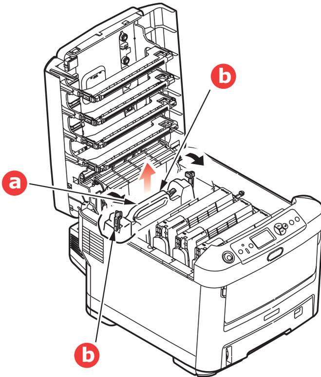
3. Pull the two fuser retaining levers (b) towards the front of the printer so that they are fully upright.
