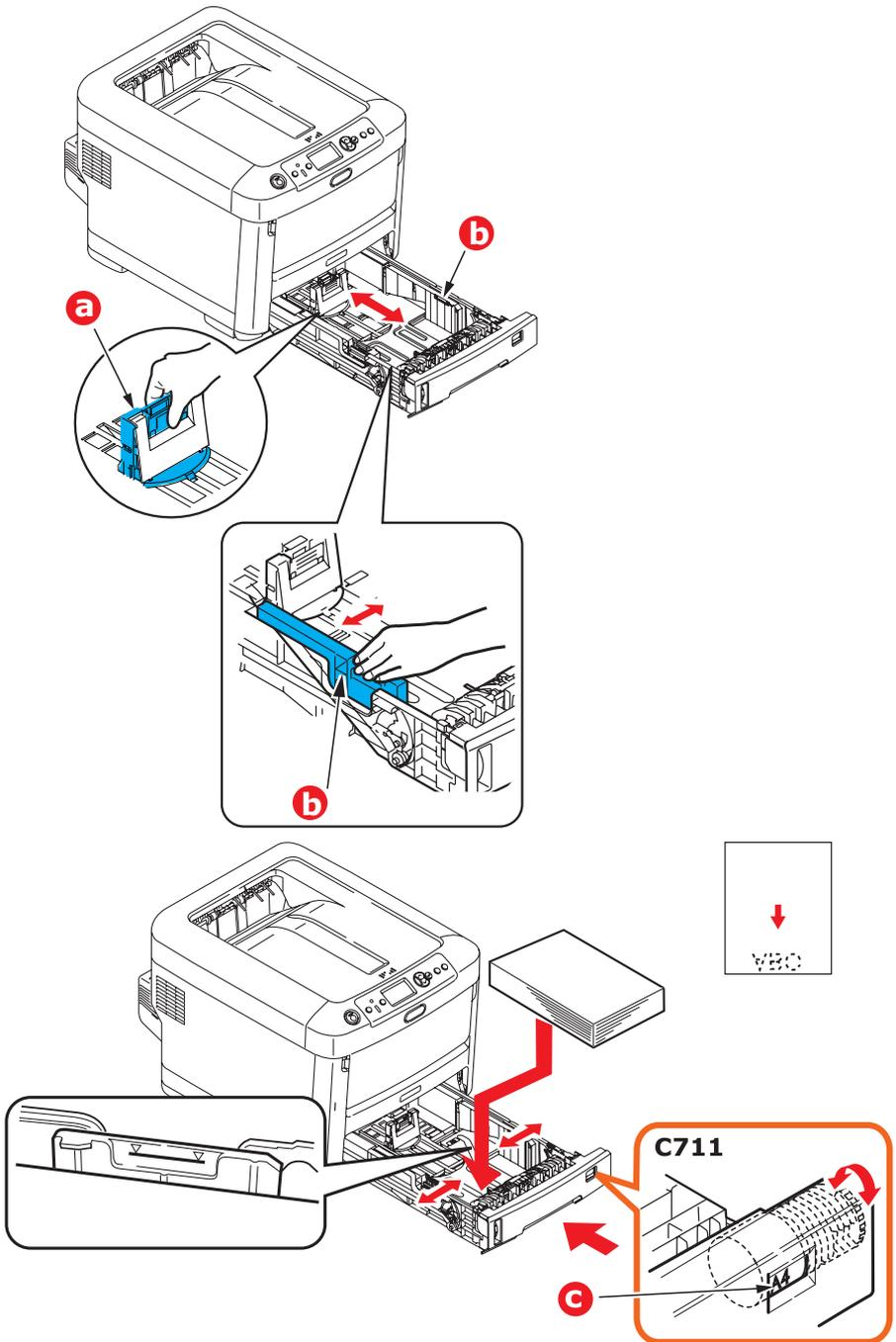
4. Adjust the rear stopper (a) and paper guides (b) to the size of paper being used.
