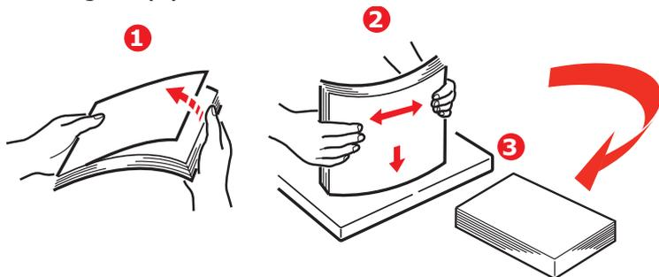
3. Load paper (letter headed paper face down and top edge towards the front of the printer), as shown.
