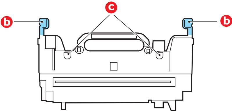
7. Lower the fuser into the printer, locating the two lugs (c) into their slots in the metal partition which separates the fuser area from the image drums.
