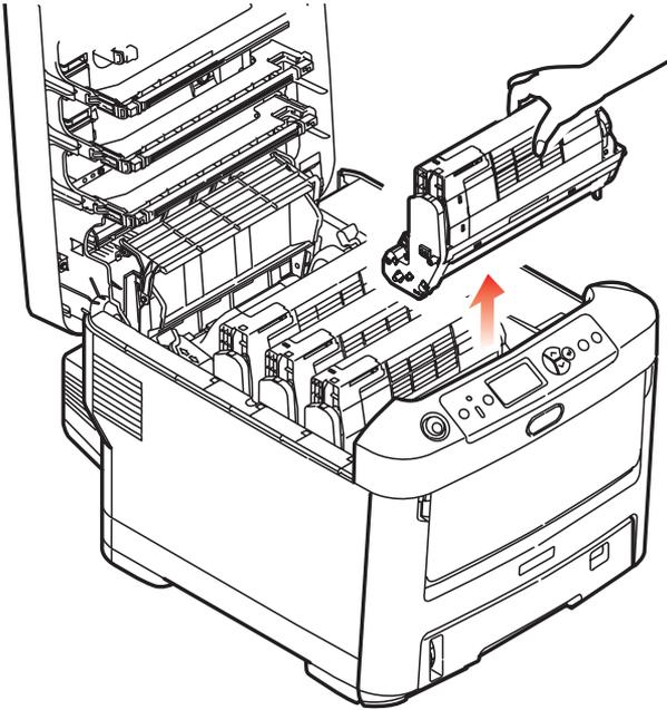
4. Put the assembly down gently onto a piece of paper to prevent toner from marking your furniture and to avoid damaging the green drum surface.
