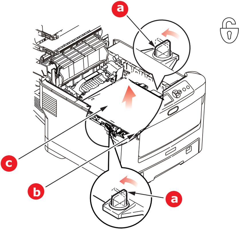
5. Turn the two fasteners 90° to the left. This will release the belt from the printer chassis.
