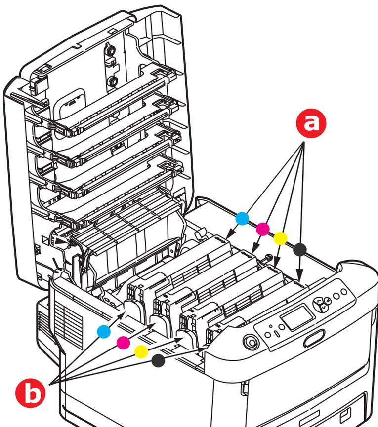
3. Lift each of the image drum units out of the printer and place them in a safe place away from direct sources of heat and light.
