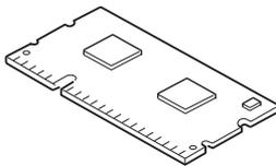
The basic printer model comes equipped with 256 MB of main memory. This can be upgraded with an additional memory board of 256 MB or 512 MB, giving a maximum total memory capacity of 768 MB.
