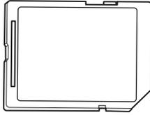
The optional SD card enables collating of printed pages and can be used to store overlays and macros, fonts, and secure or proof documents waiting to be printed.
