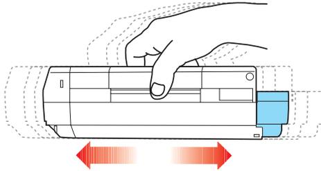
7. Remove the wrapping material and peel off the adhesive tape from the underside of the cartridge.
