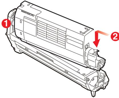
9. Push the colored release lever away from you to lock the toner cartridge onto the new image drum unit and release toner into it.
