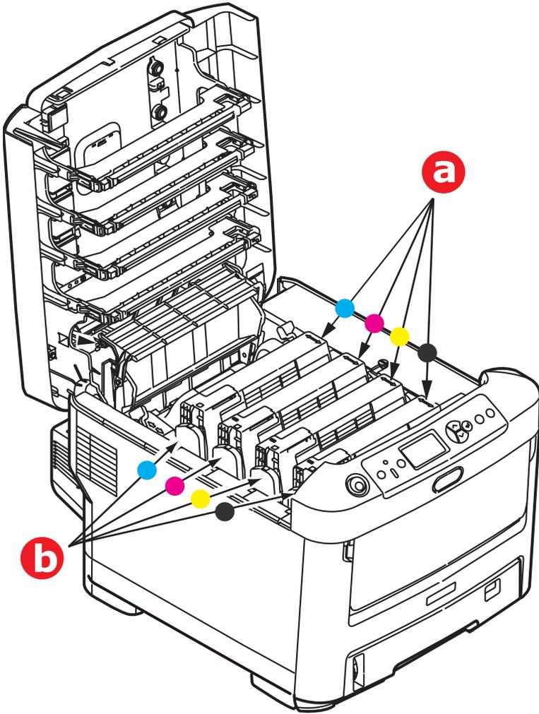
3. Holding it by its top centre, lift the image drum, complete with its toner cartridge, up and out of the printer.
