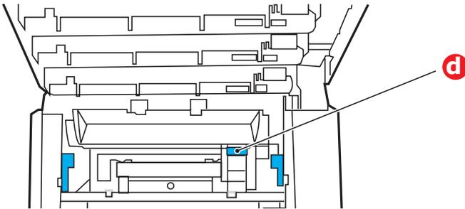
11. If you are not using the rear exit tray, close it once any paper has been removed from this area.
