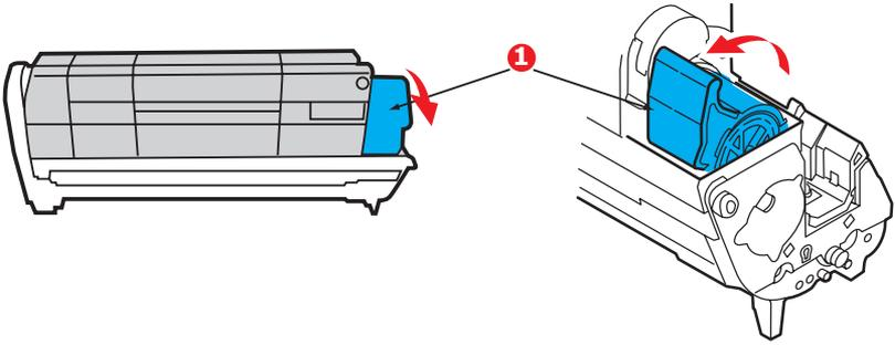
6. Lift the right-hand end of the toner cartridge (1) and then draw the cartridge to the right to release the left-hand end as shown (2), and withdraw the toner cartridge out of the image drum cartridge. Place the cartridge on a piece of paper to avoid marking your furniture.
