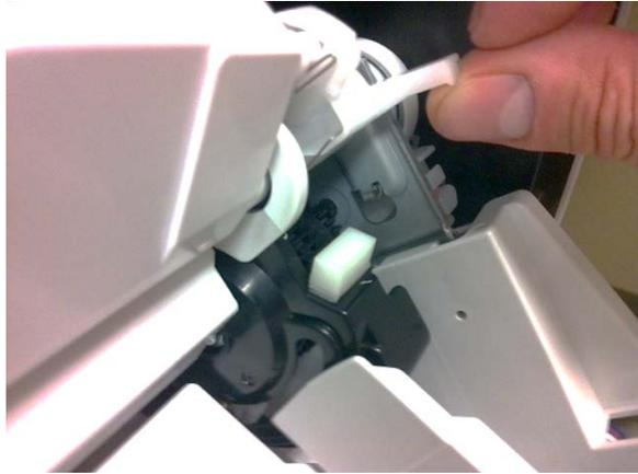
The final step is to install the wedge/spring pad assembly included with the feeder installation kit.
