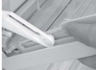
3. Flip open the top roller assembly and install reflector by peeling protective tape and adhering to area just left of the upper guide.
