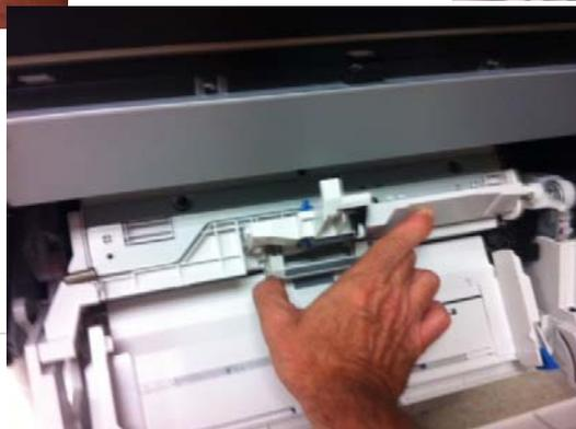
Next, install the side arm spacer to hold the lift tray in position. The spacer (either metal or plastic) has double sided tape, which helps it stay in place on the small black plastic 'shelf' on the right side of the top feed arm. Add the spacer as shown. This will hold the top roller arm all the way up when the input tray is in the closed position.
