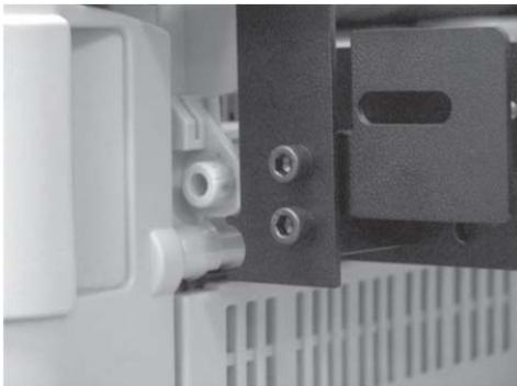
Ensure that the reflector is centered above the feeder's sheet sensor, and that the solenoid switch is centered over (and not hung up on) the paper input sensor on the printer.
