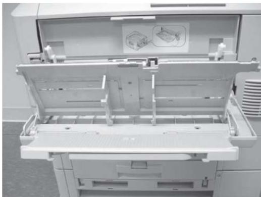
5. Locate the T-lock under the tray, remove it so that the tray can be moved and unlocked from printer chassis.
