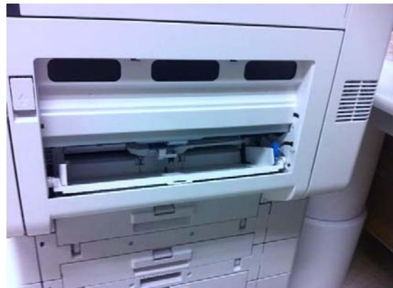
Remove the separator pad to allow media and envelopes to be more easily fed by the external feeder. First open up the input assembly and locate the top feed roller and arm. Then locate the lower center paper separator pad and remove it. This will not be needed for envelopes and media fed from the feeder.
