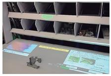
The stipulated work procedure document is projected onto the workbench by a projector installed behind
