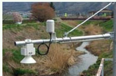
Water level indicator for measuring water at an observation point
