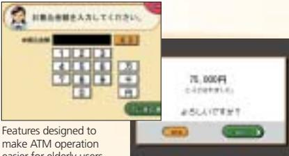
Features designed to make ATM operation easier for elderly users include large text messages, a simple flow of operations, and slow screen transitions
