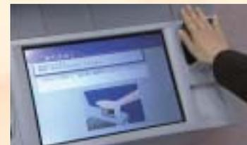
Using palm vein identification on an ATM-BankIT
