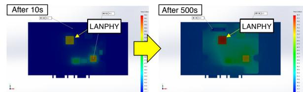
**Figure 5. Temperature Distribution Change (variable heat mass temperature)**
