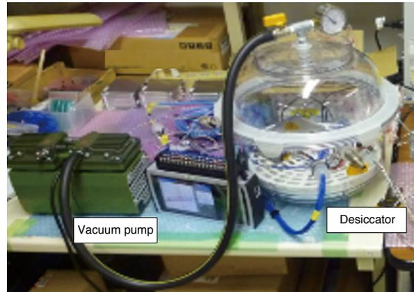
Figure 9. Setup for Temperature Rise Measurements
