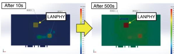
Figure 8. Temperature Distribution Change (specified heat mass temperature)
