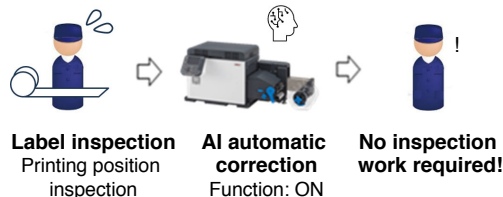
Figure 3. AI Automatic Correction of Printing Position for Small Label Printers
