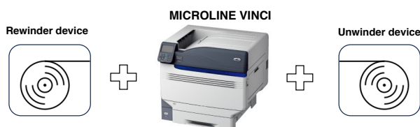
Figure 4. Built-In Modularization of A3 Color Printers
