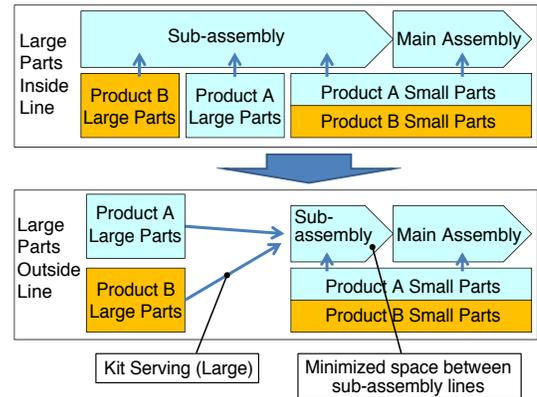
Figure 9. Modification of Large Parts Supply Method
