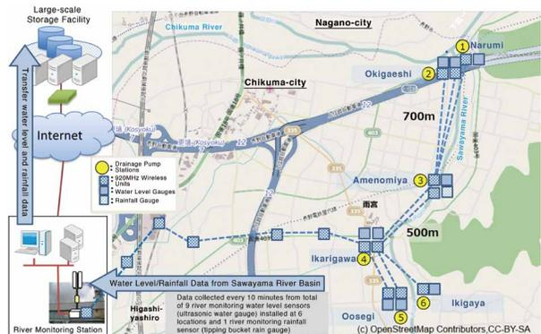
**Figure 3. Configuration of System Installed at Sawayama River, Chikuma-city**
