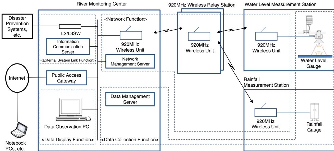
Figure 1. Configuration of River Monitoring System
