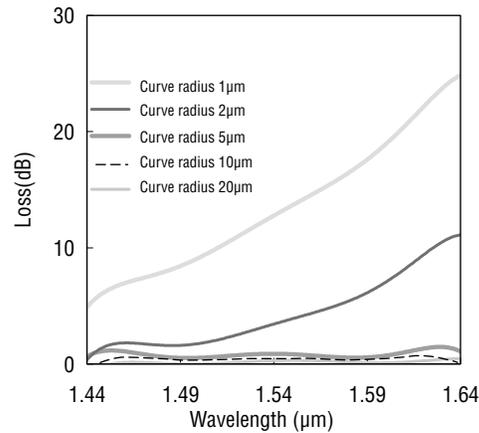
Figure 5. Loss Measurements for Curved Waveguides Curved waveguides of radius 1-20µm
