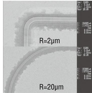
Figure 4. SEM Images of Curved Waveguides for R = 2 and 20µm
