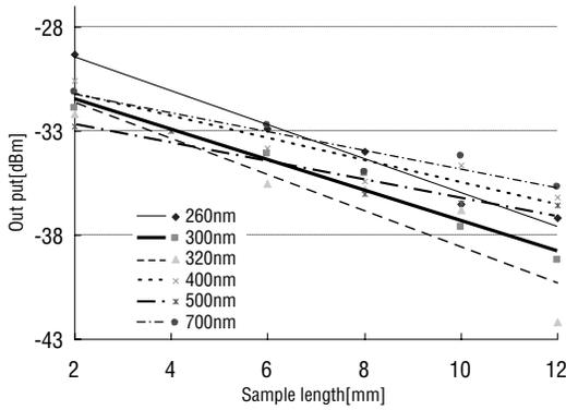
Figure 3. Straight Waveguide Propagation Losses
