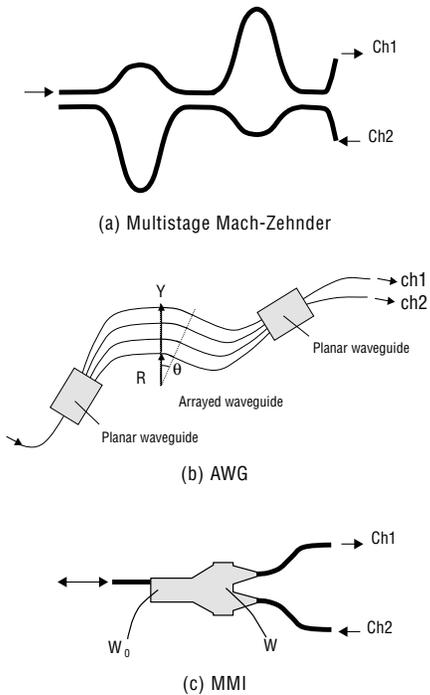
Figure 6. Overview of Wavelength Mux/Demux
