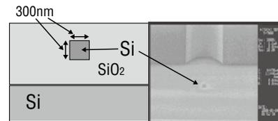
Figure 2. Actual Fabricated Silicon Waveguide
