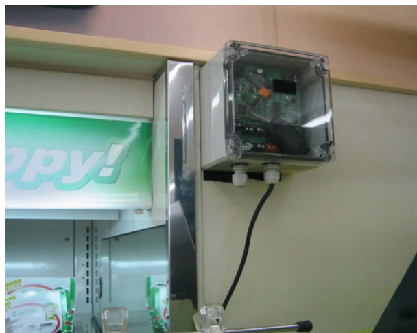
Photo 2 Wireless transmission component of wireless sensor
