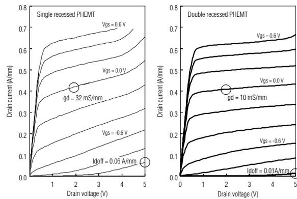
Fig. 3 I-V characteristics of PHEMT
