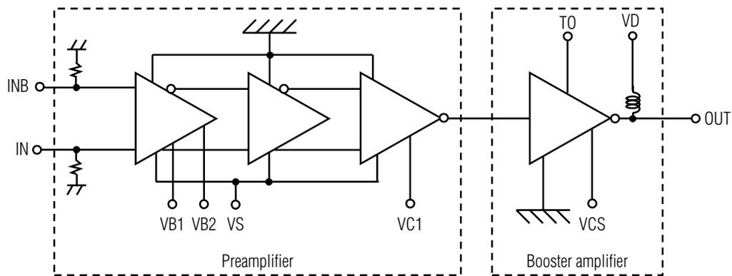
Fig. 1 Configuration of LN modulator driver
