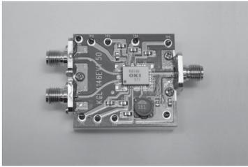
**Photo 2** Evaluation board of LN modulator driver
