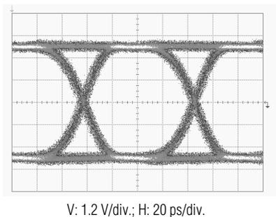
**Fig. 7** Output waveform of LN modulator driver
