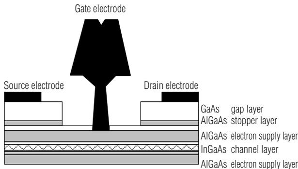
Fig. 2 Structure of double recessed PHEMT
