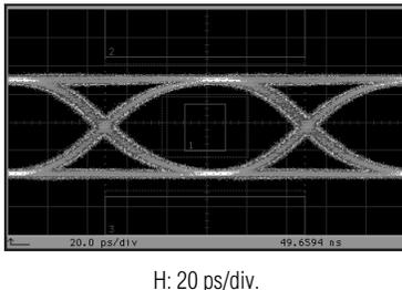
**Fig. 8** Optical output waveform for evaluation of LN modulator driver in combination with LN modulator
