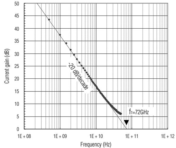
Fig. 4 High frequency characteristics of double recessed PHEMT
