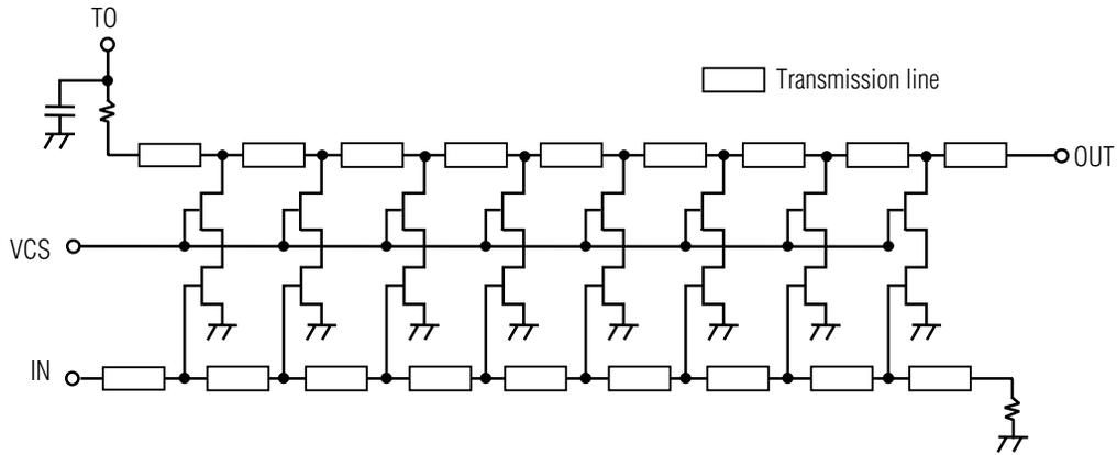
Fig. 5 Circuit configuration of booster amplifier
