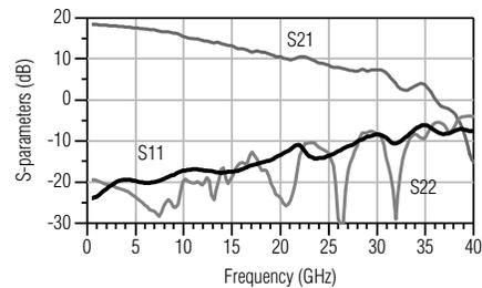
Fig. 6 S-parameter characteristics of booster amplifier
