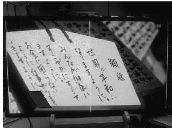
**Photo 2** Actual image on panel (right half is image with individualized gamma compensation for RGB)
