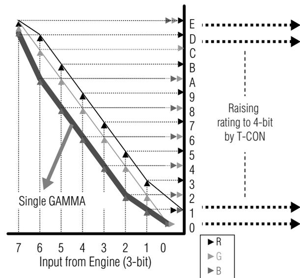
**Fig. 2** Generation of data for independent RGB gamma
