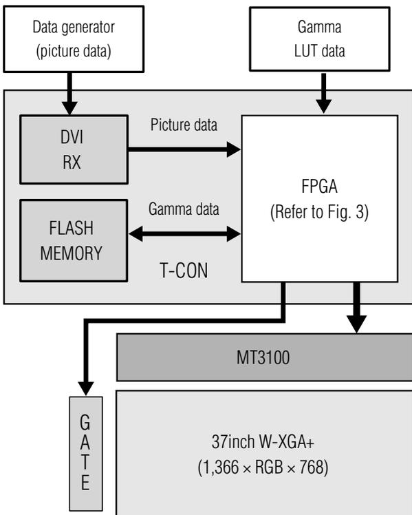
**Fig. 4** Block diagram of demonstration system
