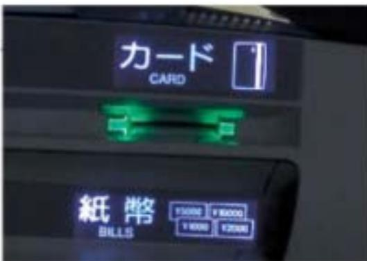
Fig. 2 Example of optical guidance
