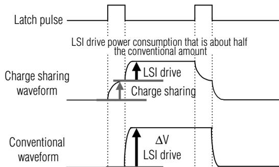
**Fig. 3 Conceptual diagram of charge sharing method**
