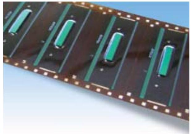
**Photo 1 Photograph of TCP mounting of ML9156**
