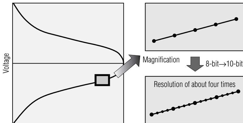
Fig. 1 Difference in display color resolutions of 8-bit and 10-bit data
