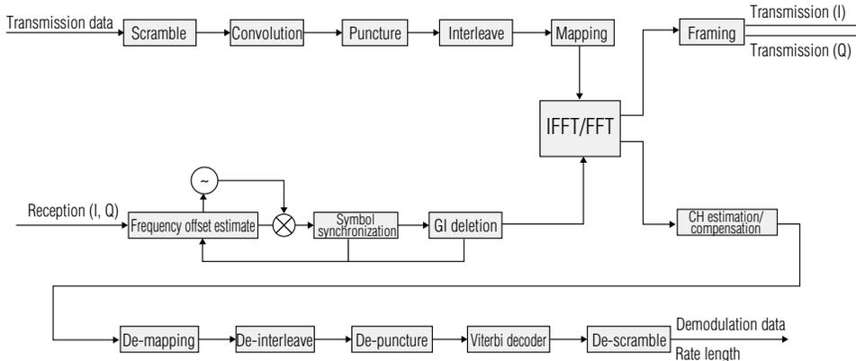
**Fig. 2 Block diagram of the 802.11a/g PHY BB signal processing IP.**
