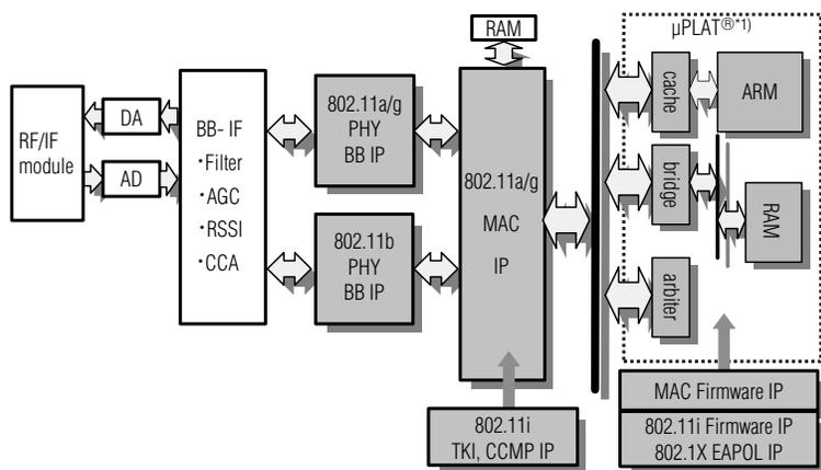
Fig. 1 Configuration example of a wireless LAN transceiver LSI.
