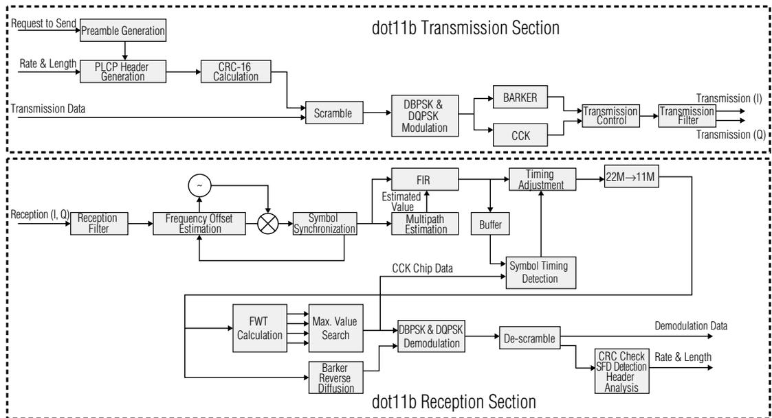
Fig. 3 Block diagram of the 802.11b PHY BB signal processing IP.
