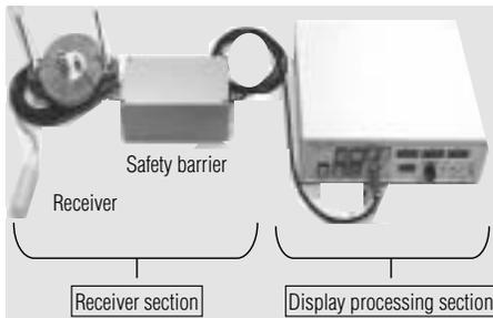
Fig. 8 Configuration of a Sonic Tester.
