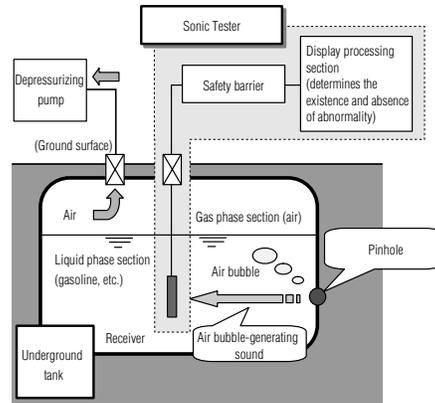
Fig. 9 Summary of an inspection with a Sonic Tester.
