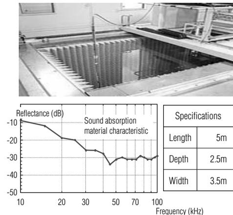
Fig. 4 Anechoic water tank.
