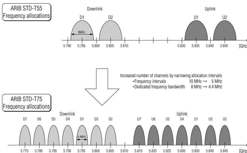
**Fig. 1 Frequency allocation for the DSRC-type RVC system**
