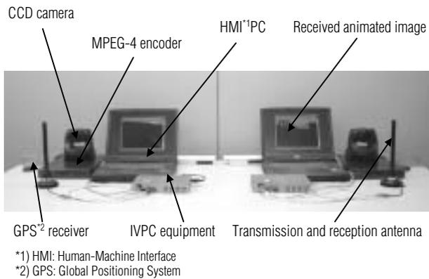
Fig. 3 IVPC system for moving image transmission
