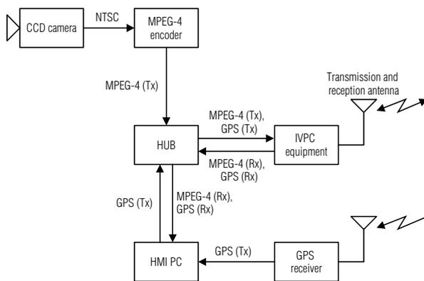
Fig. 4 System block diagram of the IVPC system for moving image transmissions
