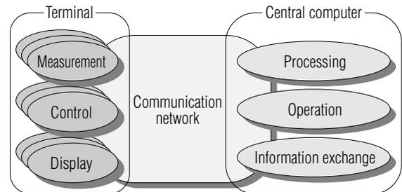
Fig. 1 Existing independent information and communication system of the road and river administrators
