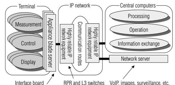
Fig. 2 Components that configure the IPGW
