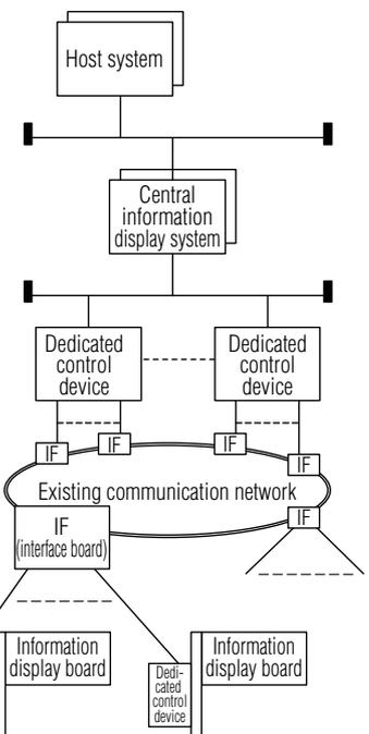
Fig. 4 Figure 4: Conventional central information display system
