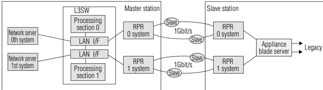
Fig. 3 Example of an IPGW redundant configuration
