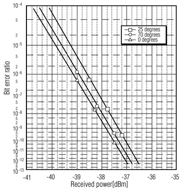
Fig. 6 Error rate characteristics
