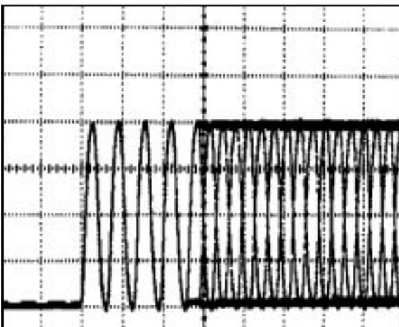
Fig. 5 155 Mb/s ONT optical output waveform
