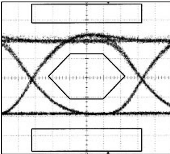
Fig. 3 155 Mb/s OLT optical output waveform
