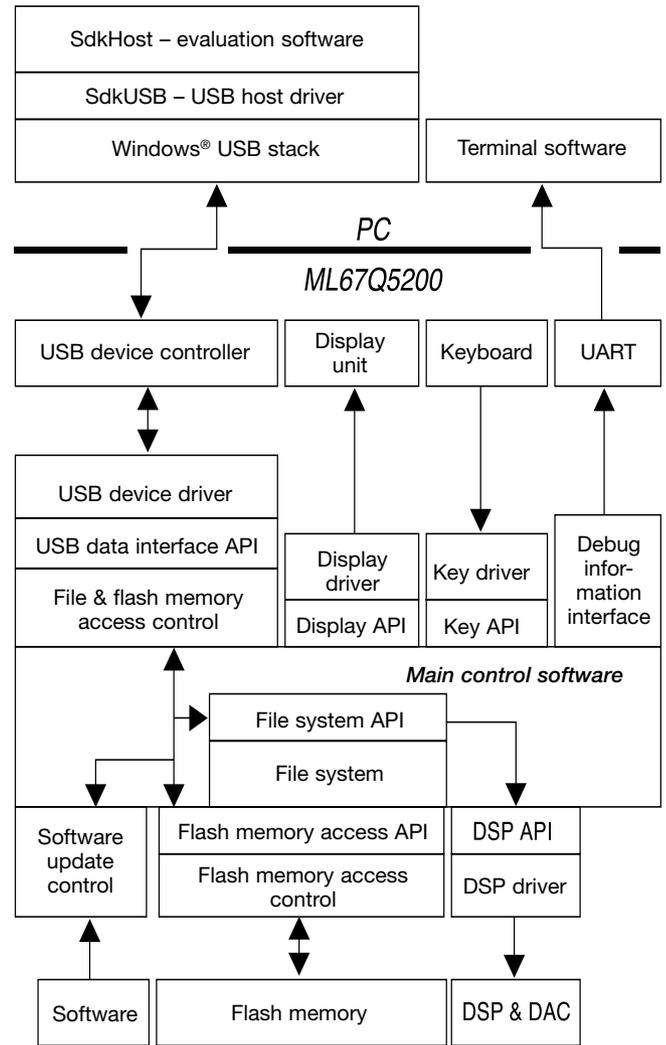
Fig. 2 Software structure
