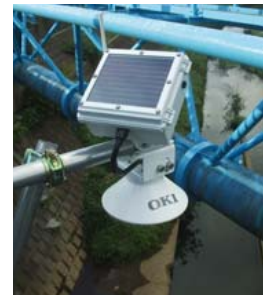
“Zero-energy ultrasonic water-level gauge”
