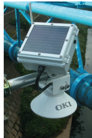
The network type “zero energy ultrasonic water-level gauge”. Wiring construction work is unnecessary due to the adoption of a wireless system and solar cell.
