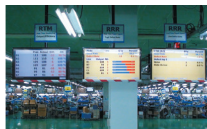
Screens of the real-time defect reporting system. When a defect occurs, the process, parts, cause, response situation etc. are displayed.
