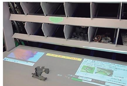
The stipulated work procedure document is projected onto the workbench by a projector installed behind the worker
