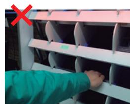
The camera and sensor behind the worker detect when the worker tries to pick from the wrong parts shelf, and the projector illuminates the shelf in red
