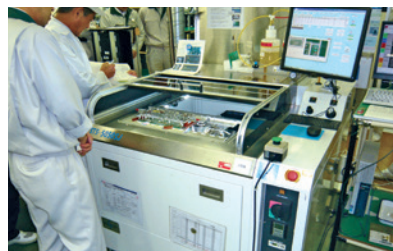
Point DIP machines that solder the exact locations necessary have reduced environmental burden by 70% at Nagano OKI
