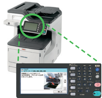
Easy-to-follow troubleshooting methods are illustrated by picture or animation on the large control panel. CO 2 emissions resulting from the dispatch of maintenance staff are reduced by linking with cloud services and smartphones
