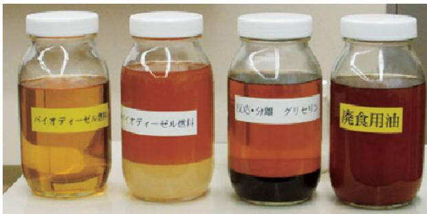
Refinement process of biodiesel fuel
