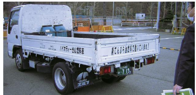
Truck running on refined biodiesel fuel
