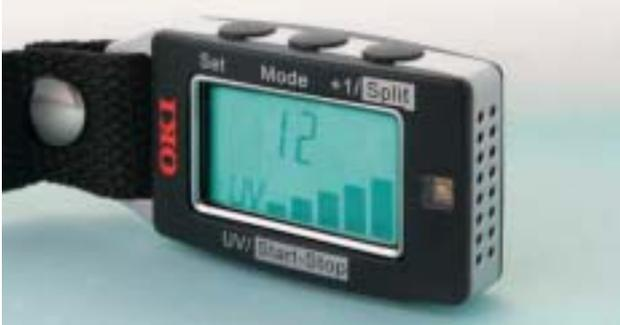
Prototype for portable accessory installing the UV sensor IC
