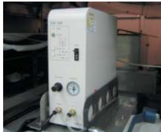
Equipment to detect impurities in lead-free solder
