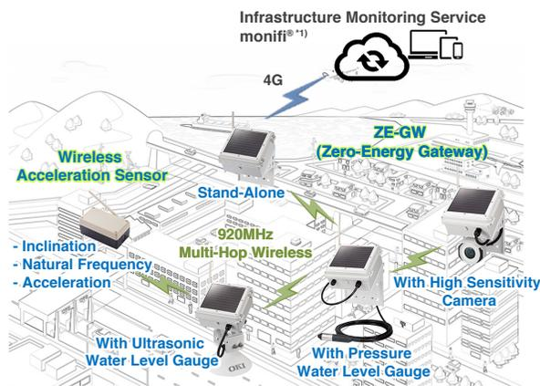
Figure 1. System Configuration
