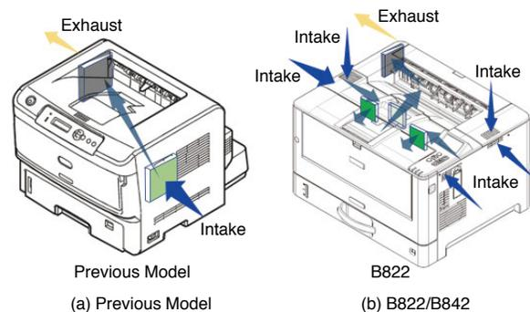
Figure 5. Internal Cooling Configuration
