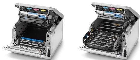
(a) Paper Jam Clearing Mode    (b) Image Drum Replacement Mode
