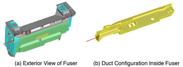
**Figure 4. Fuser Cooling Mechanism**
