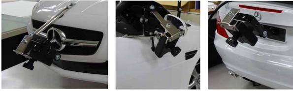
Photo 2. Camera Mounting Positions
