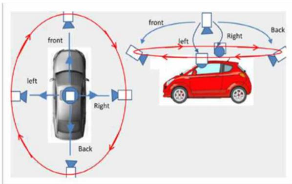
Figure 2. Virtual Camera Trajectory Diagram
