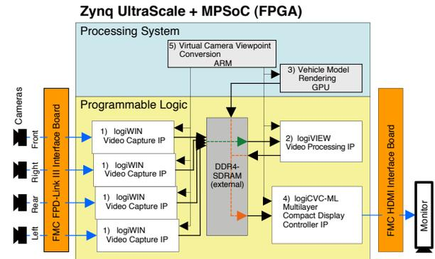
**Figure 3. FPGA and Main Hardware Components**
