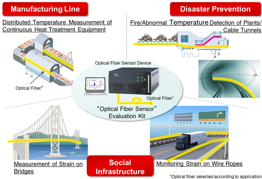
Figure 1. Areas of Optical Fiber Sensor Applications
