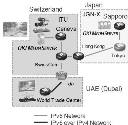
**Figure 2. I3GT Architecture at WTS-12**
