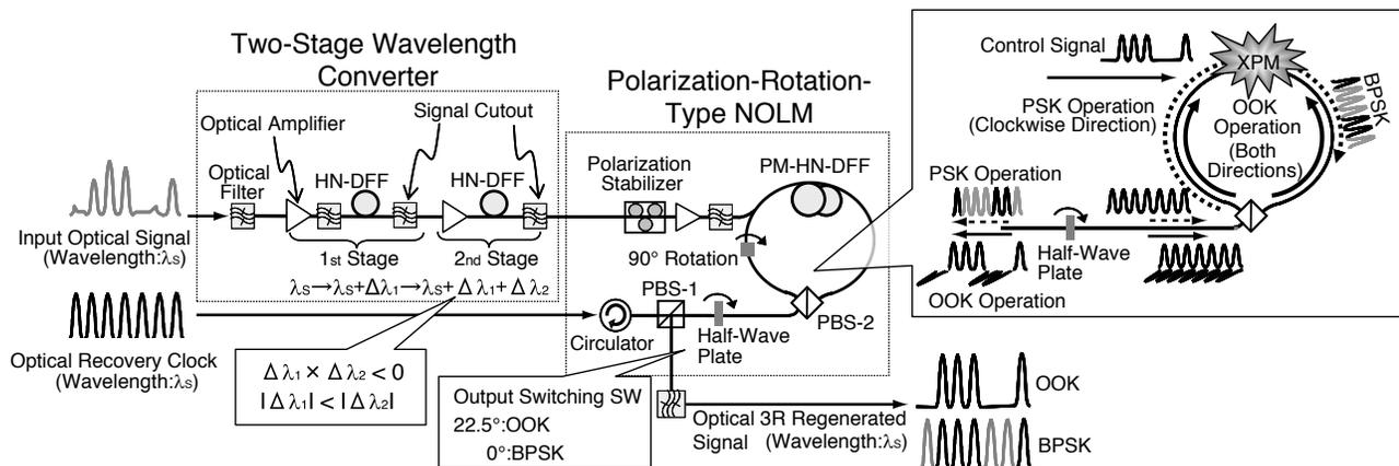
**Figure 2. Wavelength Converter with Self-Phase Modulation and Timing/Scheme Regenerator with Nonlinear Optical Loop Mirror**
