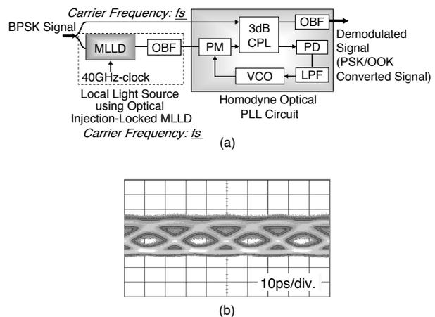
**Figure 5. (a) Homodyne Optical PLL Circuit with Optical Injection-Locked MLLD Local Light Source (b) Demodulated Waveform of 40-Gb/s NRZ-BPSK Signal**
