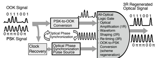
Figure 1. Configuration of a Multi-Format All-Optical-3R-Regenerator
