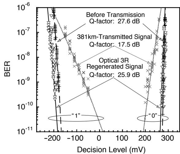
**Figure 4. Experimental Result of 160Gb/s-OOK Optical 3R Regeneration using JGNII Optical Test Bed**
