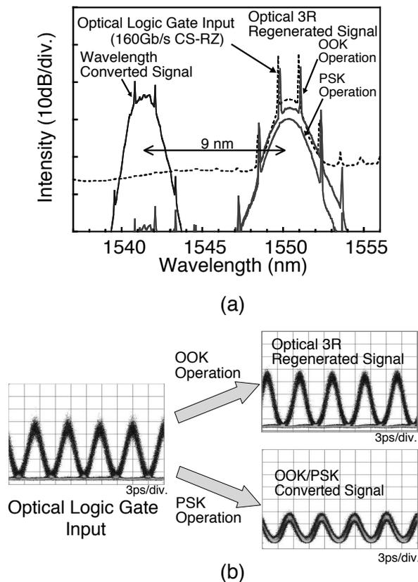
**Figure 3. 160Gb/s Optical Logic Gate Operation**
