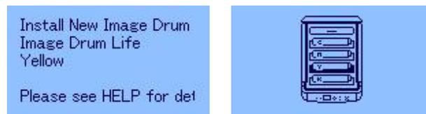
Figure 7. Error Display (two screens alternately displayed)
