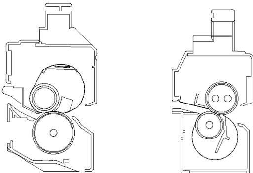
Figure 4. Cross-Sectional Comparison of Fuser Units
