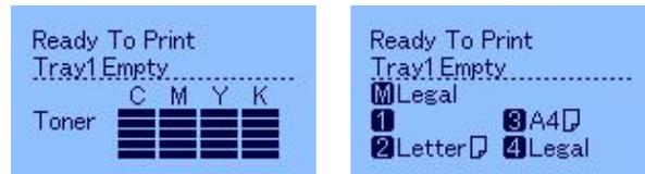
Figure 6. Standby Display (user switchable)
