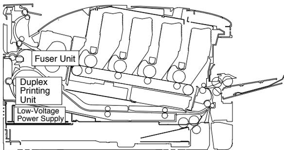
**Figure 2. C811/C831/C841 Cross-Sectional View**
