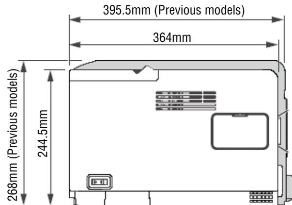
**Figure 2. Printer Size Comparison**
