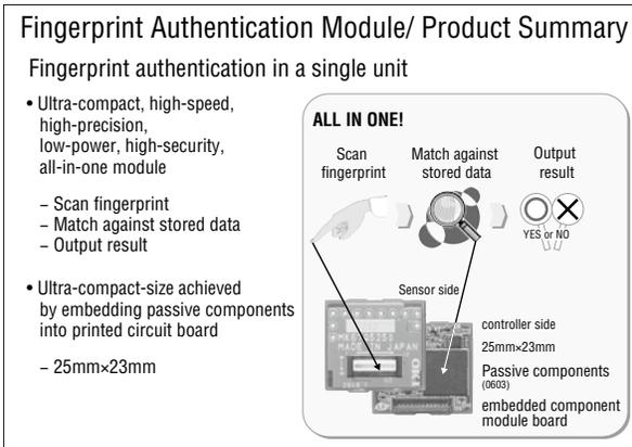
Figure 8. Fingerprint Authentication Module Board
