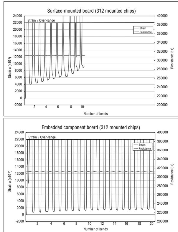
**Figure 4. Bending Reliability of Surface-Mounted and Embedded Component Boards**
