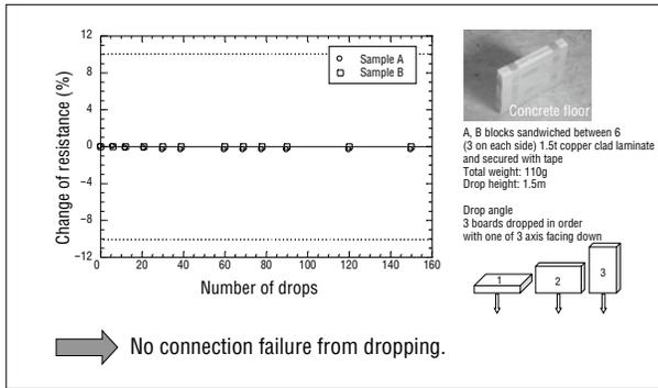
Figure 5. Result of Drop Test
