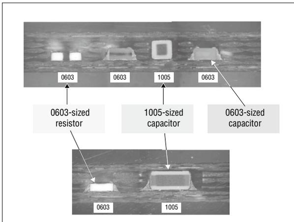
**Figure 2. Mixing Chip Components with Different Sizes**
