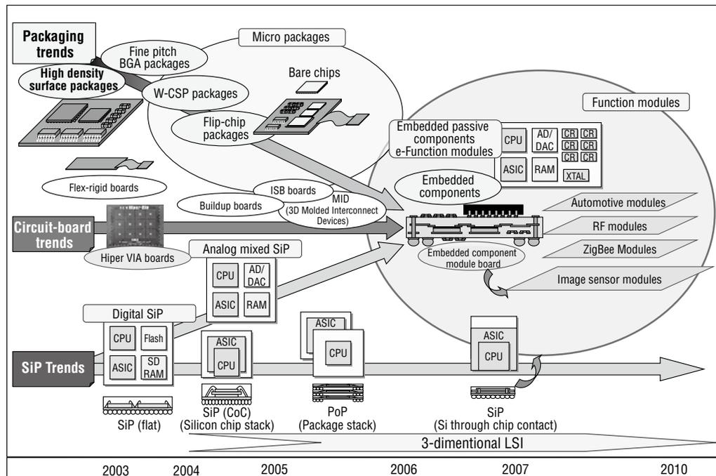
Figure 1. Trends in Printed circuit Boards and Packaging
