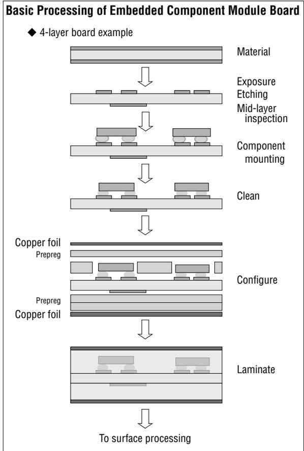
**Figure 3. Embedded Component Module Board Manufacturing**
