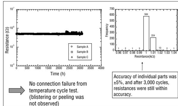
Figure 6. Result of Temperature Cycle Test
