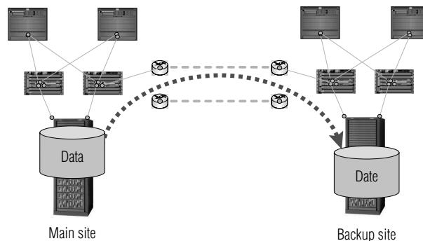
**Fig. 7** TrueCopy/SR configuration example
