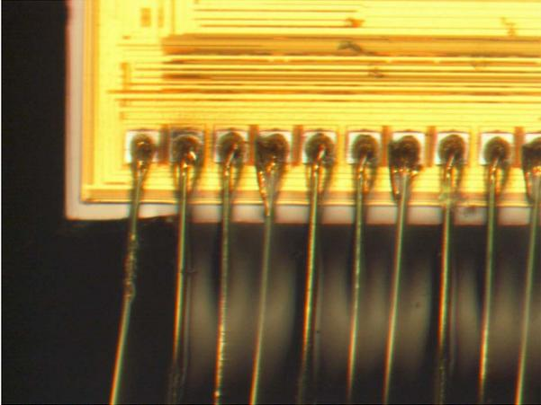
Photo 2 Example of pad wiring on a single side
