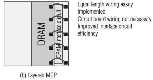
**Fig. 1** Examples of MCP configurations for chips with pads on two sides
