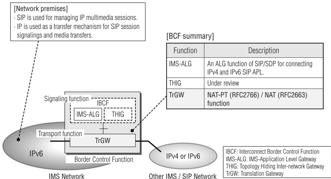
Fig. 1 Standardization of border control functions in 3GPP
