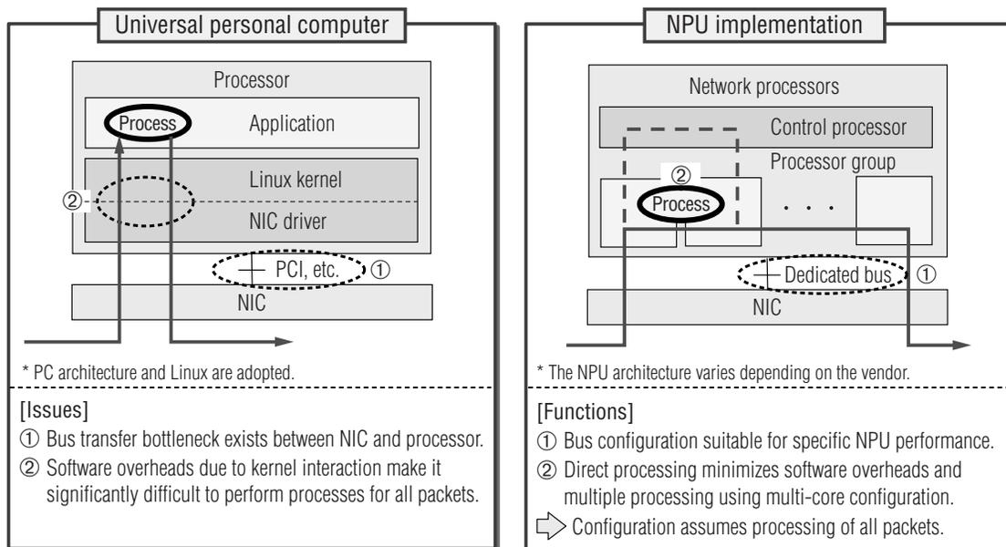
**Fig. 2 Differences between modes using universal personal computers and network processors**
