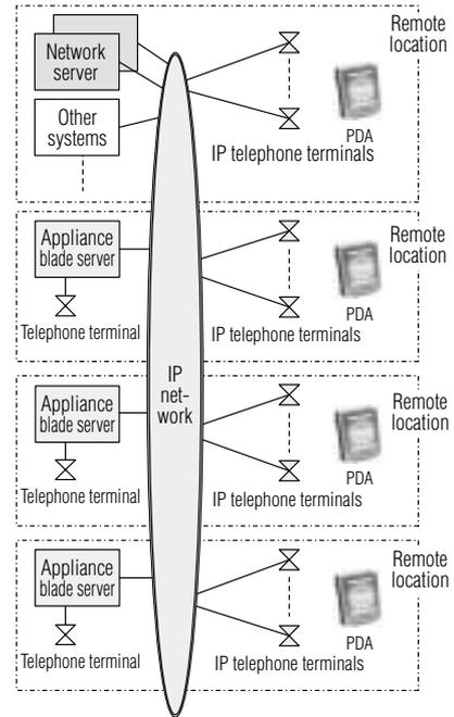
**Fig. 7 Solution for converting telephone exchange equipment**
