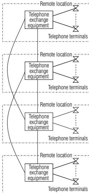
**Fig. 6 Conventional telephone exchange equipment**
