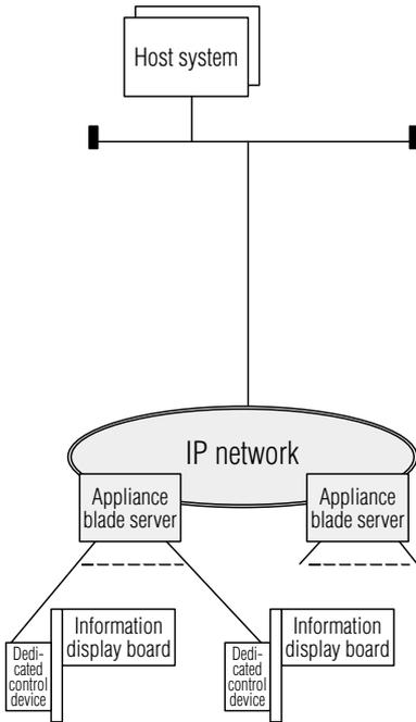
**Fig. 5 Solution for converting a central information display system**
