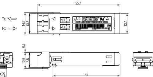
Fig. 11 External view of SFP short wavelength optical transceiver (Duplex-LC)
