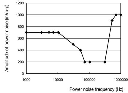
Fig. 13 Power noise tolerance
