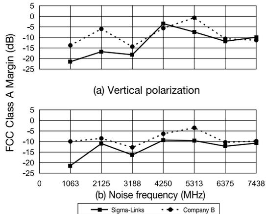
Fig. 5 Radiated noise from HBA (measured of frequency (1 GHz)
