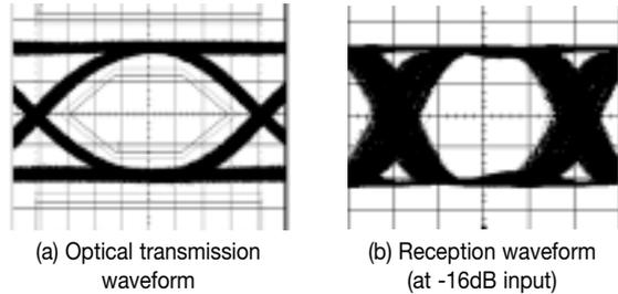
Fig. 3 Transmission and reception eye patterns (2.125 Gb/s, PRBS 2<sup>7</sup>-1, mark rate 1/2)
