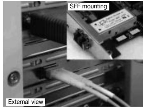
Fig. 4 Example of SFF optical transceiver in use
