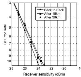
Fig. 9 Minimum optical reception power
