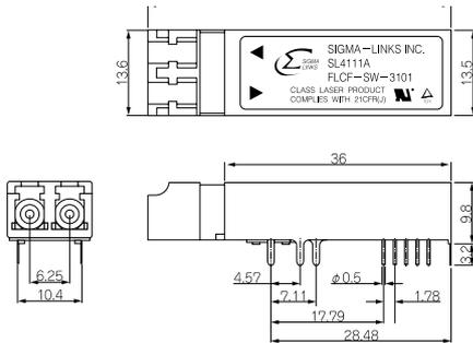
Fig. 2 External view of SFF short wavelength optical transceiver
