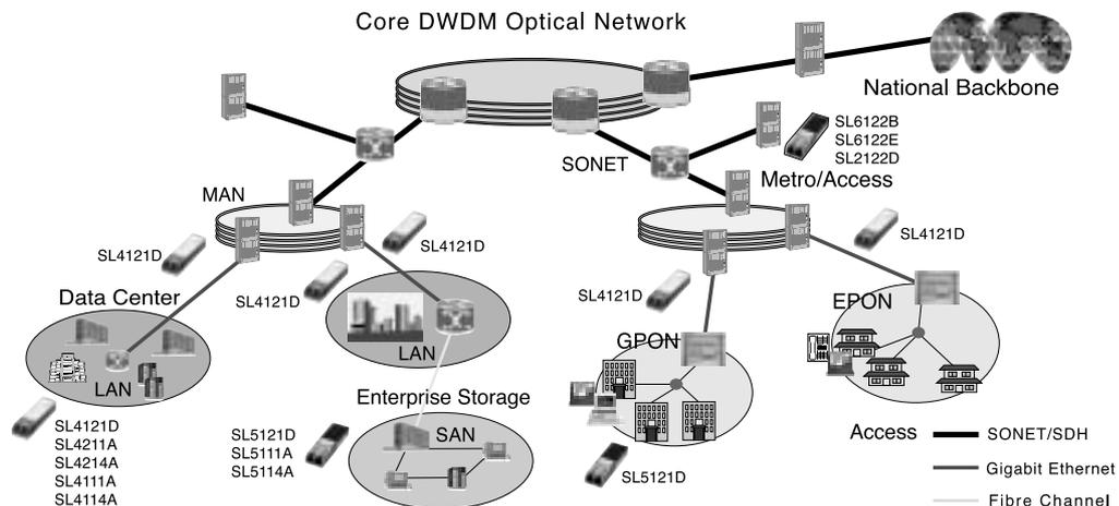
Fig. 1 Optical communications network for the broadband era
