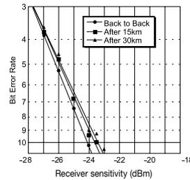
Fig. 9 Minimum optical reception power
