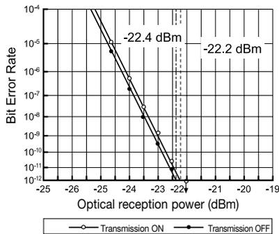
Fig. 12 Minimum sensitivity characteristics
