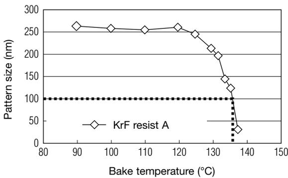
Fig. 3 Relationship between pattern size and bake temperature
