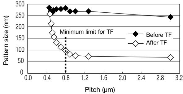
Fig. 5 Relationship between shrink dimensions and pattern pitch
