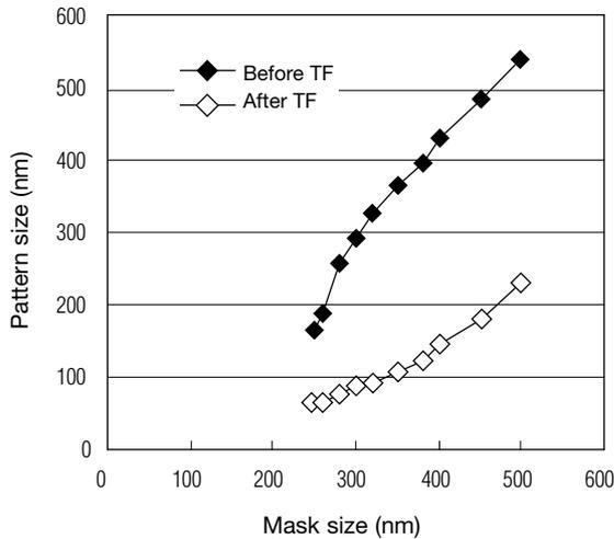
Fig. 6 Relationship between shrink dimensions and pattern size
