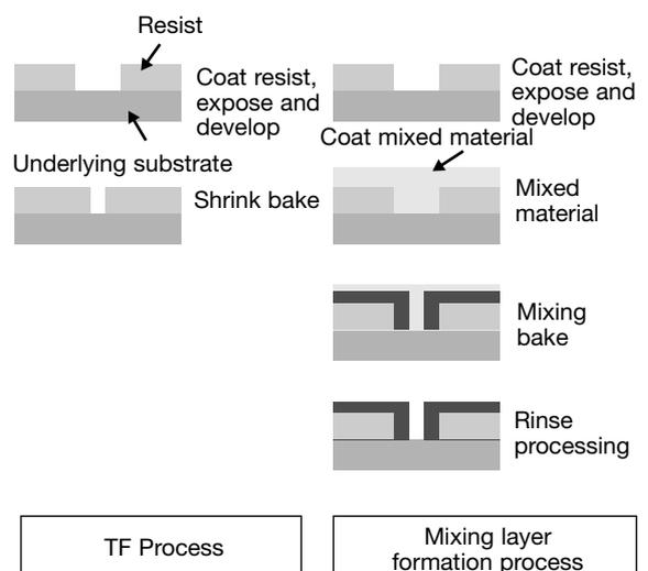
Fig. 1 Process flows of TF and mixing layer formation processes
