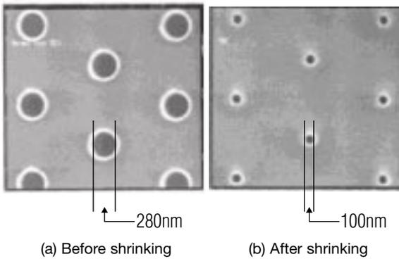
Fig. 2 Pattern size before and after shrinking
